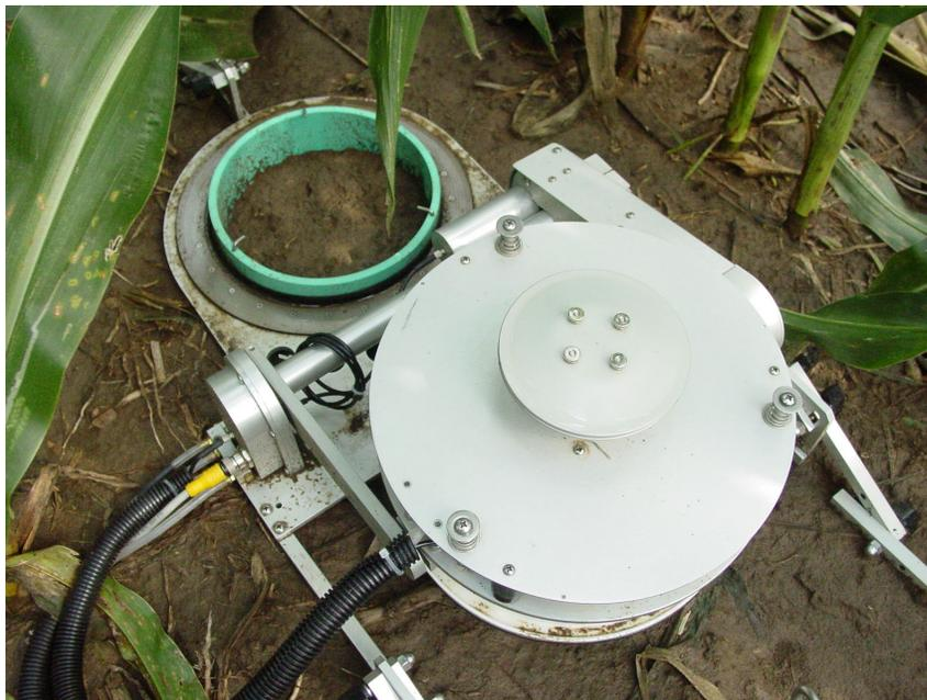
Figure A7. LI-8100 automated soil CO<sub>2</sub> flux system set up in the irrigated corn field site 1 (courtesy of LI-COR, Inc.) in ARDC, Univ. of Lincoln, Nebraska, 2006. The system consisted of an analyzer control unit and a long-term chamber (model 8100-101), collecting soil CO<sub>2</sub> data continuously for over a month (as presented in Fig. A1).
