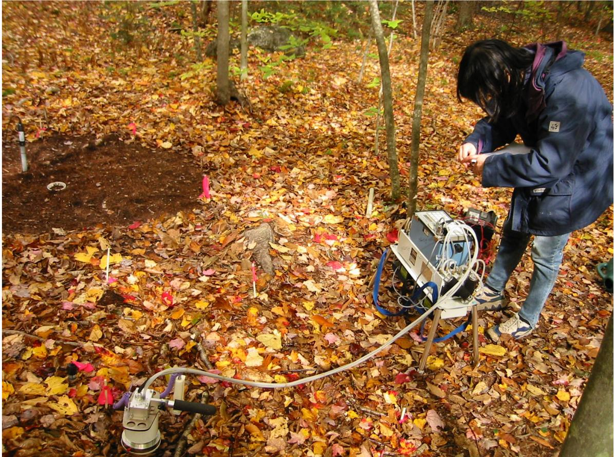
Figure A3. Field set-up and flux measurement at Harvard Forest, 2004. LI-6200 was used for CO<sub>2</sub> flux measurement here. Flux measurement was being made on a forest floor plot, while soil moisture probe was already set to prepare for measuring soil moisture on a nearby bare plot at the next time step.
