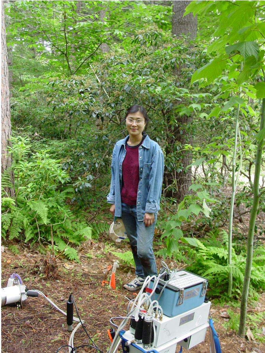
Figure A2. Field set-up at Great Mountain Forest, 2002. LI-6200 was used for CO<sub>2</sub> flux measurements. The plot shown here is a bare plot on a gentle slope.
