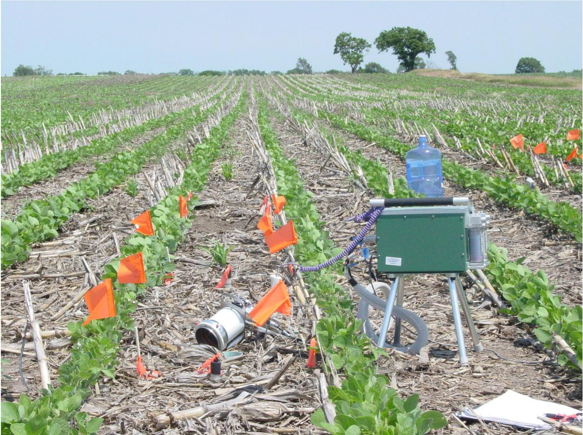
Figure A5. Field set-up at Nebraska soybean site 2, 2006. LI-6400 was used for CO<sub>2</sub> flux measurement here. Plots were placed between rows of soybean plants. The picture was taken at the beginning of the growing season (June 20).
