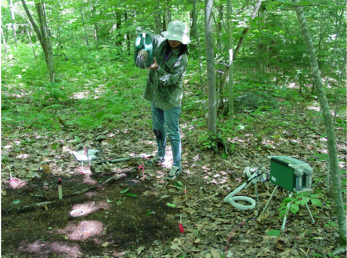
Figure A4. Field set-up and rain simulation at Harvard Forest, 2005. LI-6400 was used for CO<sub>2</sub> flux measurement here.
