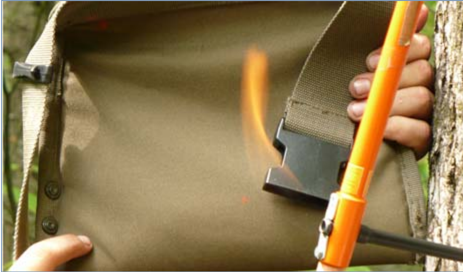
A flame fueled by methane shoots out of an oak tree being cored at Yale Myers Forest.
